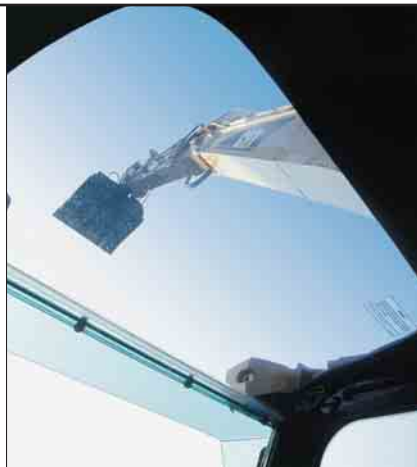
Skylight. A unique large polycarbonate skylight provides very good upward visibility, especially useful in above ground applications.
