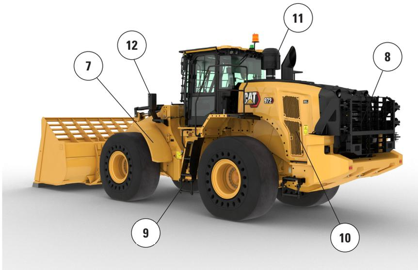
7. Narrow front steel fenders help to keep the windshield clean and are set inboard of the outer edge of the tire for added protection
