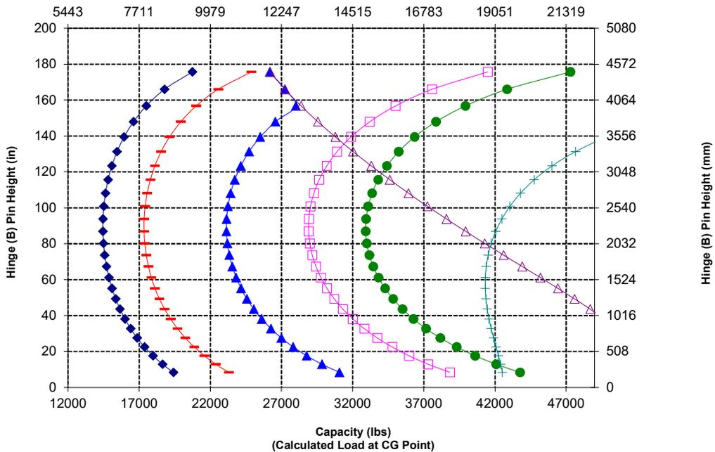
NOTE: Static tipping loads and operating weight are based on the following loader configuration: Bridgestone VJT L3 Tires, Air Conditioning, Ride Control, Powertrain Guard, Full Fluids, Fuel Tank, Coolant, Lubricants, and Operator.
