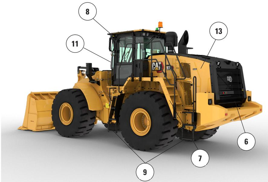
6. Ground-level parking brake override and engine shutdown switches
