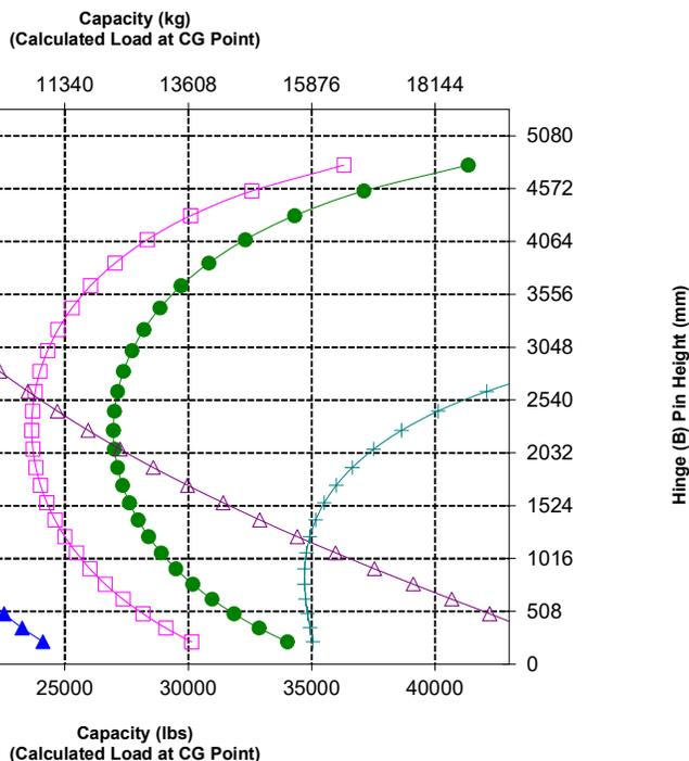
NOTE: Static tipping loads and operating weight are based on the following loader configuration: Bridgestone VJT L3 Tires, Air Conditioning, Ride Control, Powertrain Guard, Full Fluids, Fuel Tank, Coolant, Lubricants, and Operator.
