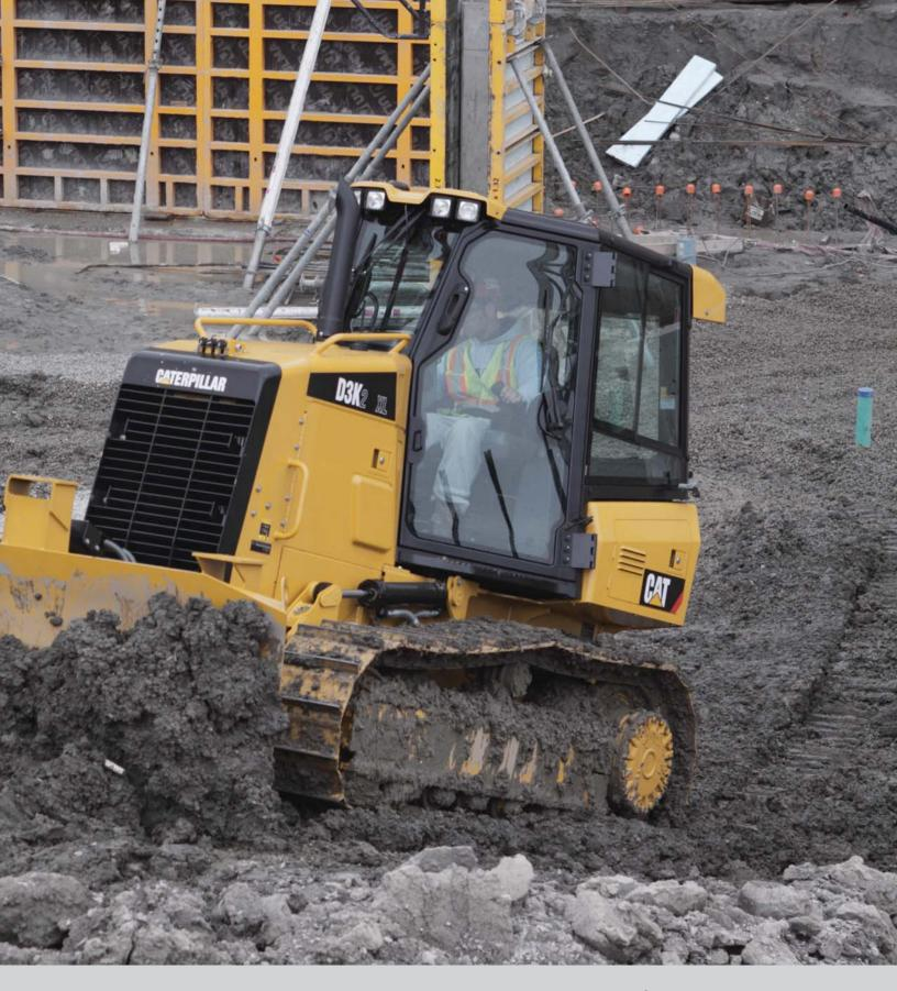
Experience the most intuitive finish grading tractor in the industry. The Cat® D3K2 Track-Type Tractor with Stable Blade delivers a smooth finish grade with less operator effort. Stable Blade senses ground conditions and works with the operator to produce the desired grade. The addition of the integrated AccuGrade™ grade control system helps you get to target grade even faster, with fewer passes and less manpower. From the first cut to finish grade, the D3K2 sets the standard.
