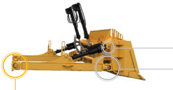
Replaceable push-arm trunnion bearing inserts
